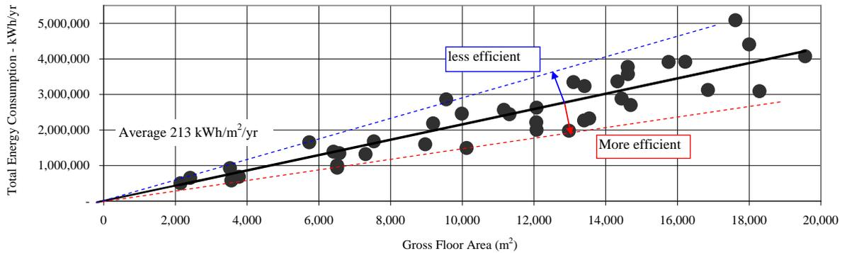
**Figure 9: Total Energy Consumption versus Gross Floor Area**
