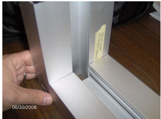
PHOTOGRAPH 9: With the sealed unit remove discontinuity of the glazing pocket at junction of the jamb and the sill shown by the red arrow.
