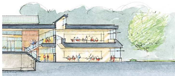
Figure 16: Building section through the south facing classroom wing and roof monitor and light well
