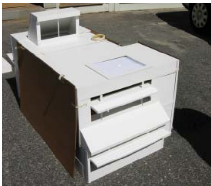
Figure 11: Daylighting Scale Model
