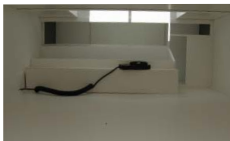
Figure 12: Daylighting Scale Model & Light meter (typical upper level south facing classroom looking north)
