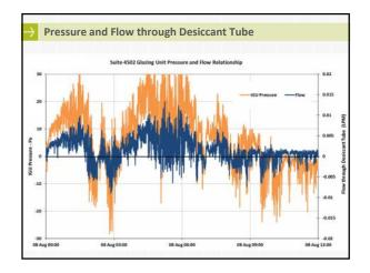
→ Air flows from outside into the IGU through edge seal defects then into suite through desiccant tube – driven by wind pressure differences and thermal expansion/contraction
