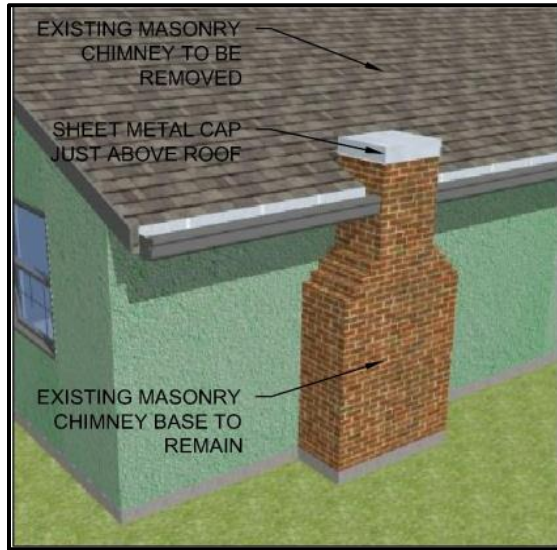
Figure 3: Dwelling with a chimney capped at the roof line.
