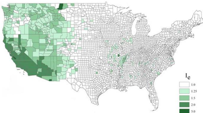
**FIGURE 2.** Maximum strength and stiffness factor  $I_e$  to exceed 2015 IBC and IRC seismic design requirements where the incremental benefit remains cost-effective.
