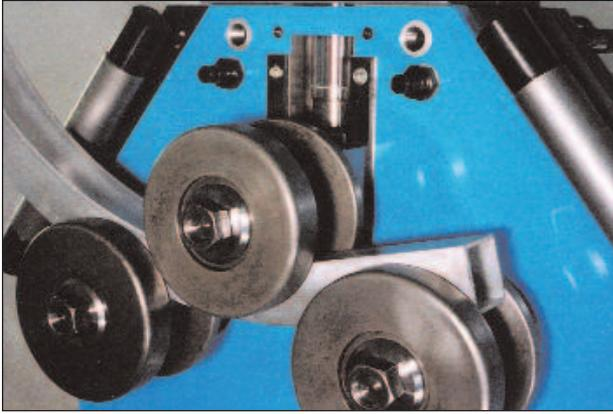
**Benders like this Promaco Model RBM 2-40H can accommodate a wide variety of dies for different shapes and materials. The machine also accepts custom dies for nonstandard applications.**
