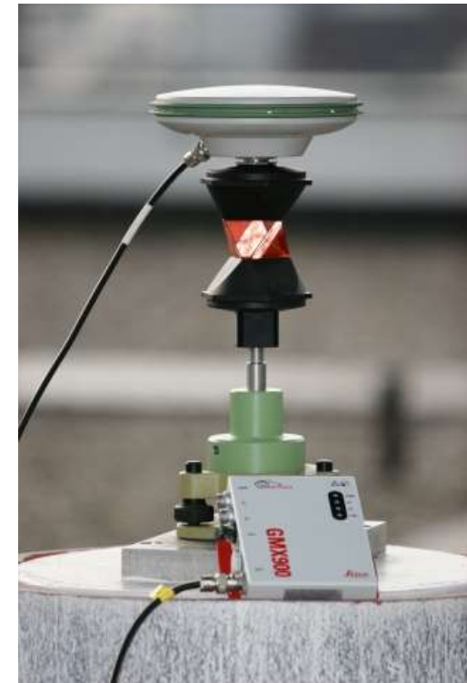
Reflector with 5/8" thread adapter for mounting of GPS antenna.
