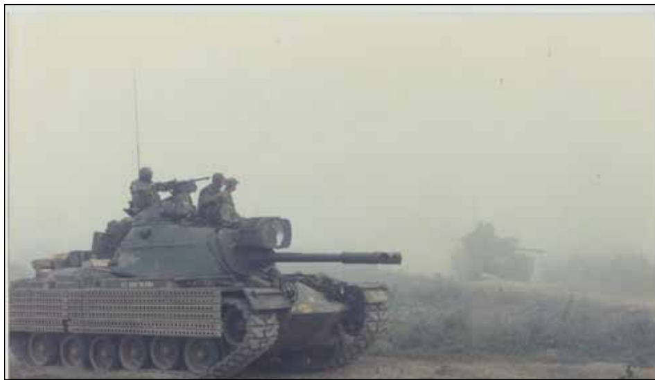
C Troop tank, Vietnam, late 1967-early 1968, with RPG plate protection on the side. Photo courtesy of Dwight W. Birdwell
