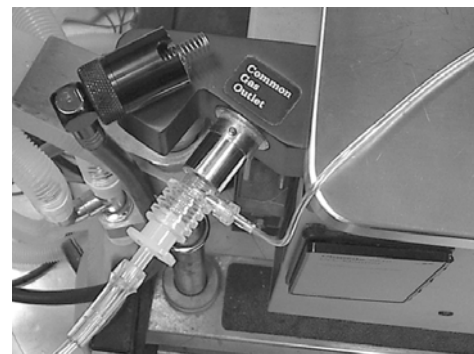
Figure 3. A nasal cannula mated to a common gas outlet via a 5-mm endotracheal tube connector and a gas sampling connector with a gas sampling line attached. From: Lampotang: Anesth Analg, Volume 101(5), November 2005.1407-1412
