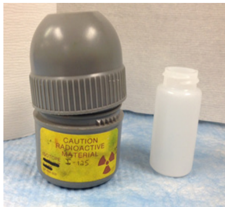
[Fig. 7] The seed is placed in a vial and stored in a lead pig until disposal by radiology.
