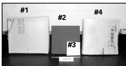
All samples were initially 12" x 12" and exposed to 200°F for 7 days:
