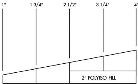
**TYPICAL CROSS-SECTION OF 3/16" SLOPE
