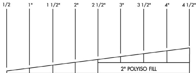
**ABBREVIATED PANEL: TYPICAL CROSS-SECTION OF 1/8" SLOPE
