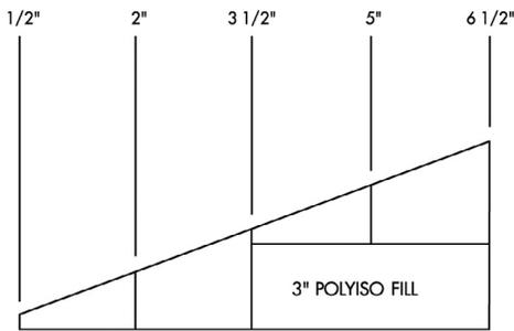
**TYPICAL CROSS-SECTION OF 3/8" SLOPE
