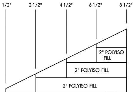
**TYPICAL CROSS-SECTION OF 1/2" SLOPE
