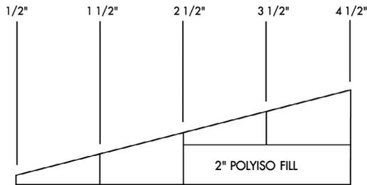
**ABBREVIATED PANEL: TYPICAL CROSS-SECTION OF 1/4" SLOPE
