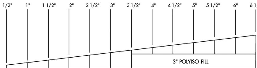
**EXTENDED PANEL: TYPICAL CROSS-SECTION OF 1/8" SLOPE
