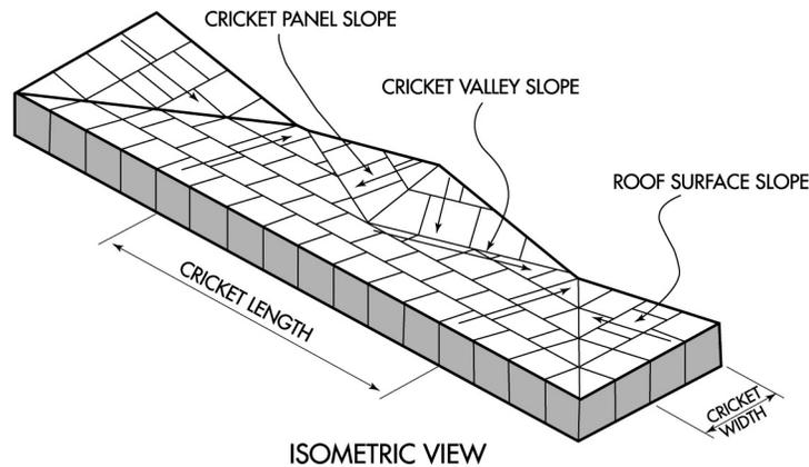
**Rise** is the roof surface slope x 1/2 the cricket width (C to E)
