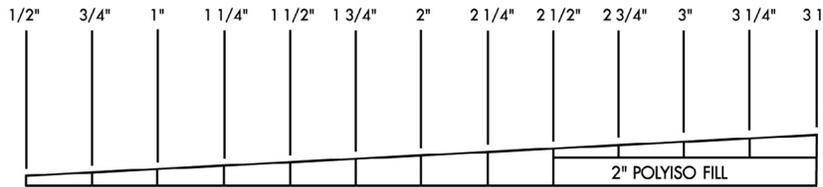
**TYPICAL CROSS-SECTION OF 1/16" /FT. SLOPE
