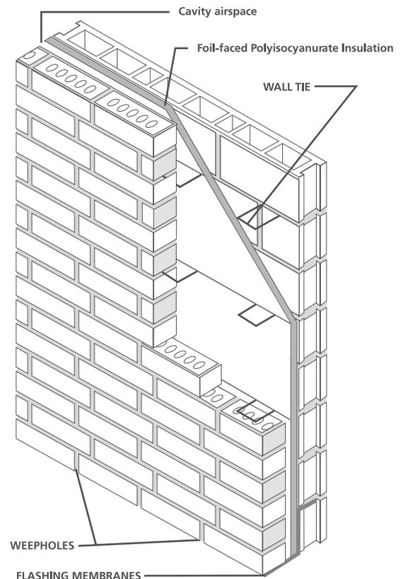
amount of moisture that does penetrate seeps primarily through microscopic cracks between the masonry and mortar bond and down the cavity face of the outer wythe. Organizations that provide cavity wall design details recommend an unobstructed air space. This air space allows the moisture to seep to the lowest level where wall flashings direct the moisture back to the building's exterior via weep holes. As stated by the Masonry Advisory Council:
