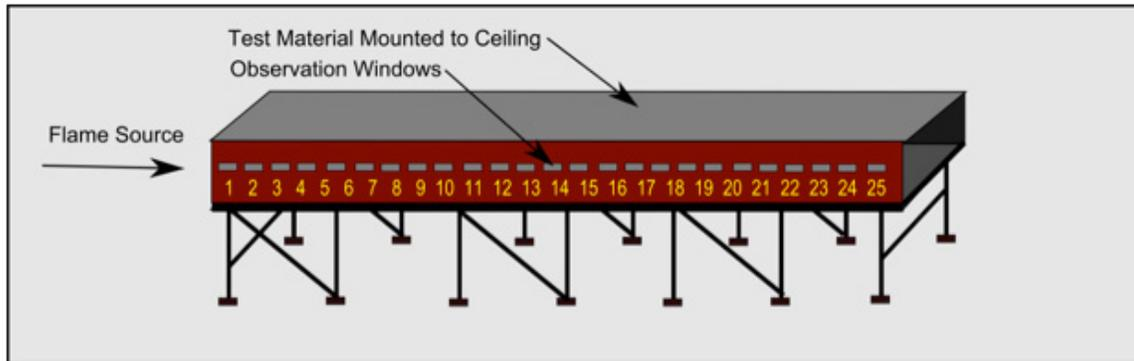
**The Steiner Tunnel (ASTM E-84) test consists of a 25' vented tunnel lined with firebrick. The test material is mounted to the top of the chamber. At one end of the chamber, the sample is subjected to a high-energy flame for ten minutes. Flame spread is determined visually through windows built into the tunnel. An optical cell mounted at the tunnel exhaust measures smoke density. (Illustration by TEGNOS Research, Inc.)**
