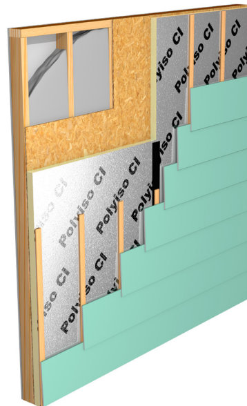
Figure 1. A typical residential wood-frame wall constructed with OSB sheathing and Polyiso CI.
