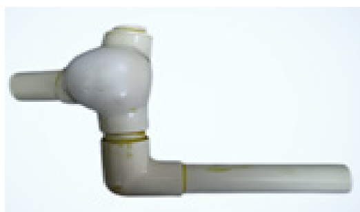
Images 20 and 21. Excess Cement in Fitting Damage
