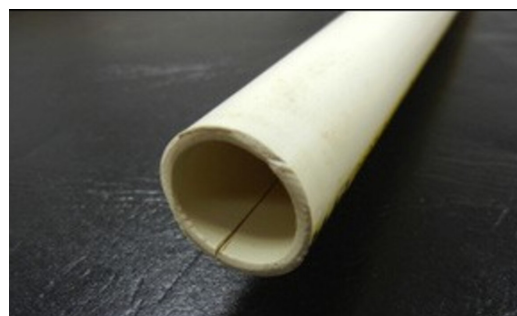
Image 17. Damaged Tubing End
