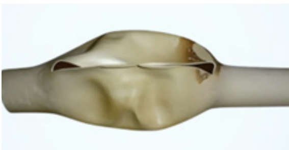
Image 24. Excessive Temperature and Pressure Damage
