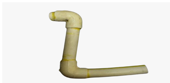
Image 7. Pipe Under Excessive Flexural Stress
