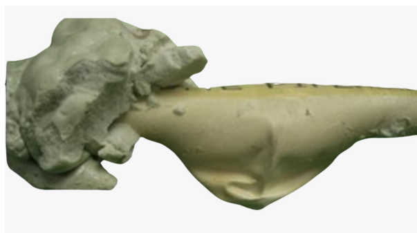
Image 3. Excessive Heat Damage Caused by Installation of Two-Part Spray Foam
