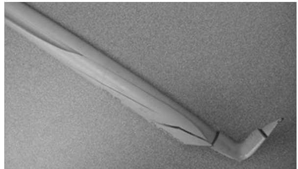
Image 25. Examples of Damage Resulting From Freezing
