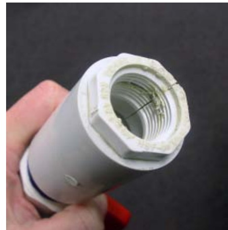
Figure 10: Over tightened connection caused the female adapter to split.
