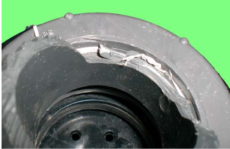
Figure 9: Vibration failure of male threads.
