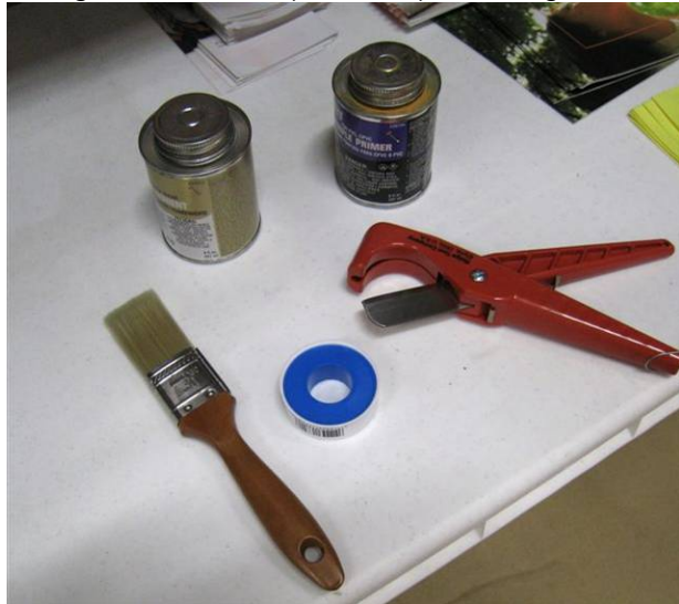
Figure 30. PVC Requires Simple Joining Tools
