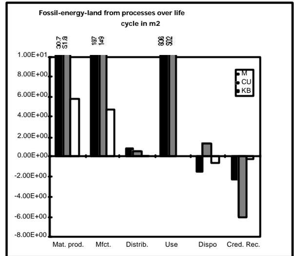
**Fig. 3** Land-space from process energy (Monitor, Control Unit, Keyboard).
