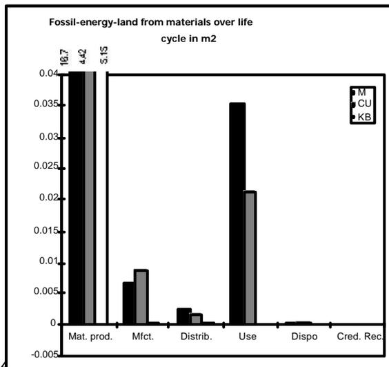
**Fig. 2** Land-space from materials energy (Monitor, Control Unit, and Keyboard).
