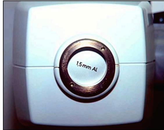
Figure 5. 1.5 mm of Aluminum Filtration
