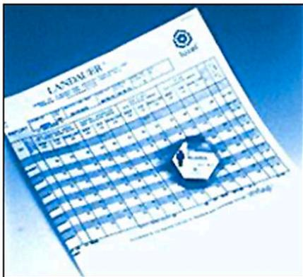
**Figure 9.** Stimulated Luminescence Dosimeter
