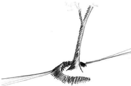
Figure 6: Verge around the tree that catches the water Source: Joubert, 2007a: own drawing
