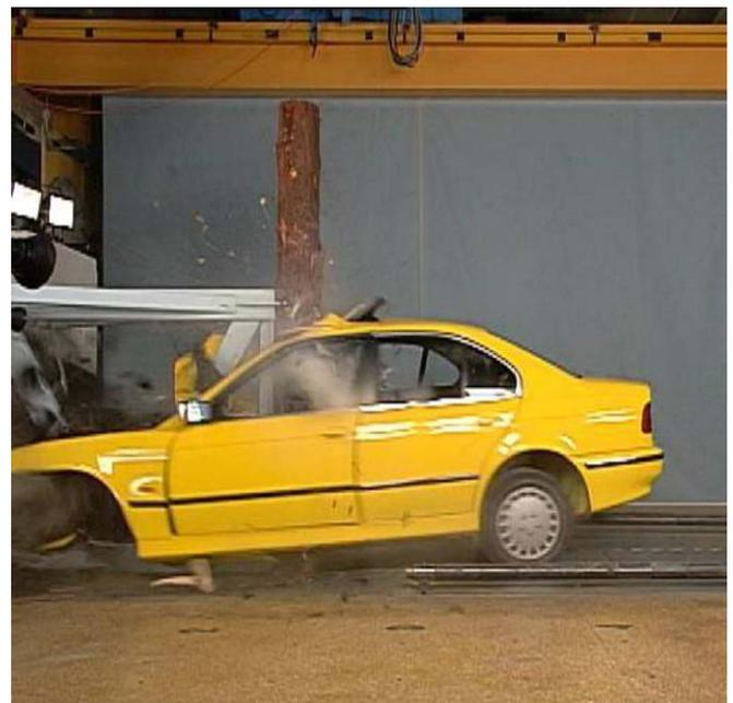
Fig. 4. A simulated collision into a tree. The picture shows the approximately position of the tree after a 70 km/h crash.
