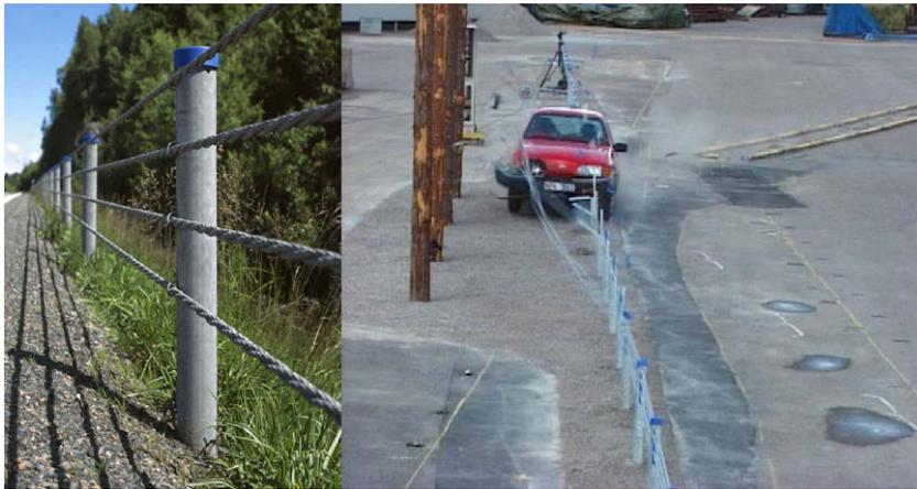
**Fig. 6.** Different cable-barriers used as side barriers.
