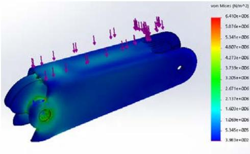
Figure 12 Finite Element Analysis of the Middle Finger Proximal Phalanx.
