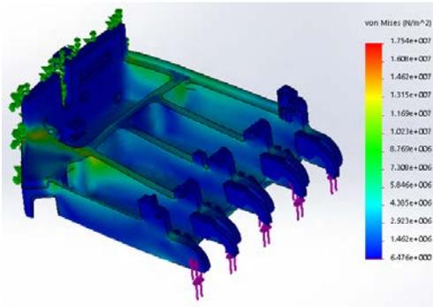
Figure 11 Finite Element Analysis of Palm.
