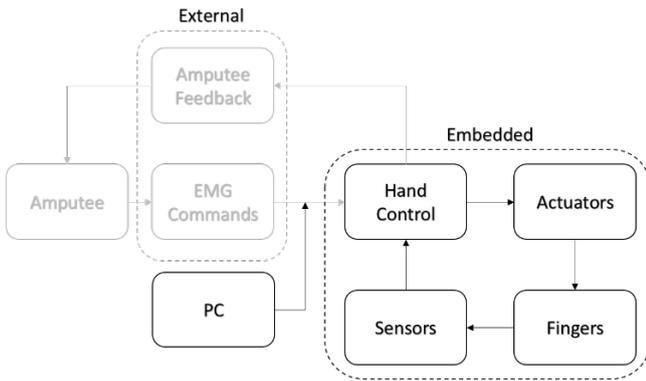
Figure 8 Overview of Hand Control via the PC.
