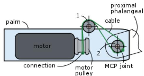
Figure 3 Pulley Finger Mechanism Concept.
