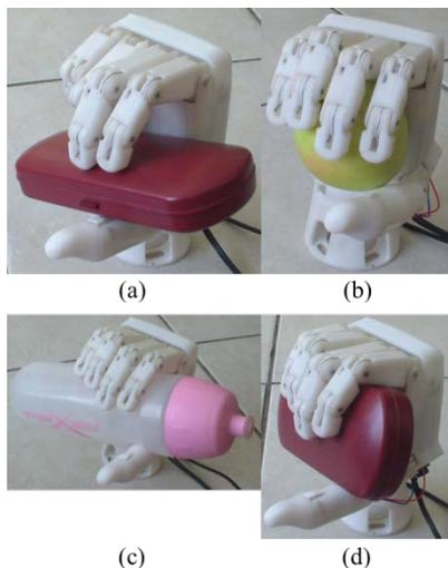
Figure 16 Grasping Objects; (a) glasses case grasp 1, (b) apple, (c) water bottle, (d) glasses case grasp 2.
