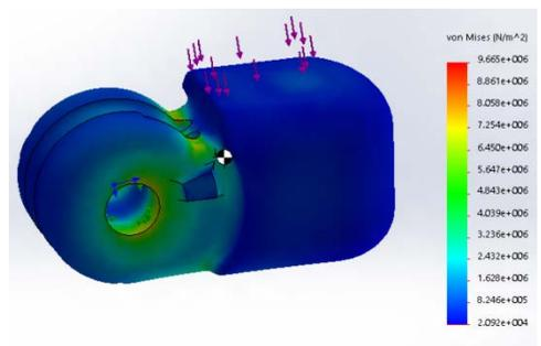
Figure 14 Finite Element Analysis of the Distal Phalanx.
