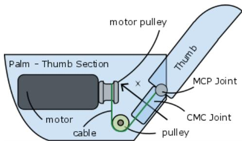
Figure 4 Thumb Pulley CMC Joint.
