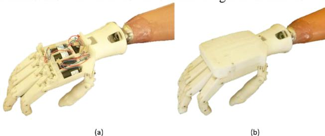
Figure 6 Constructed Hand: (a) without top cover or electronics, (b) with top cover.
