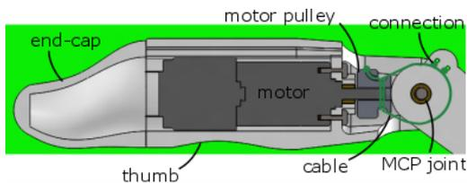
Figure 5 Thumb Pulley MCP Joint (Cross-Section).
