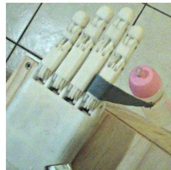
Figure 17 Finger Load Test (Top View).
