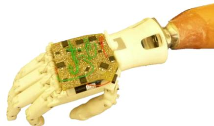
Figure 7 Physical Right Hand with Electronics.
