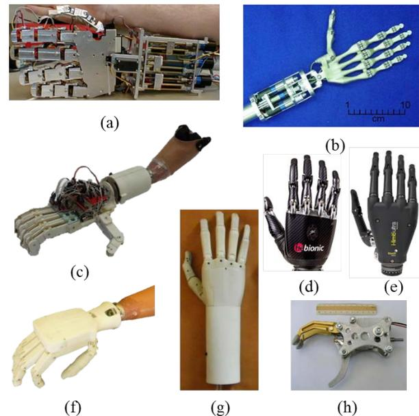
Figure 19 Visual Comparison of the hands in table 4; (a) [12], (b) [14], (c) Touch Hand I, (d) Bebionic3 [15], (e) I-limb Ultra Revolution [3], (f) Touch Hand II, (g) [11], (h) [13].
