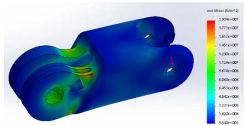
Figure 13 Finite Element Analysis of the Middle Finger Middle Phalanx.
