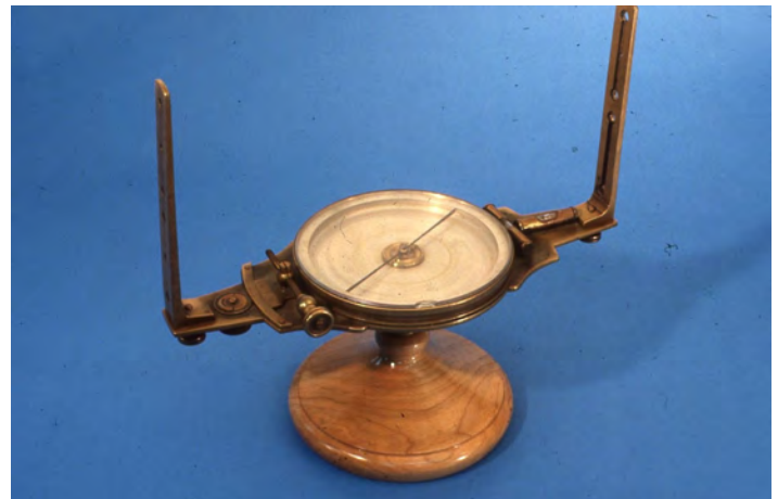
The standard American vernier compass by W. & L.E. Gurley. This form with vernier, outkeeper, sights, level vials, was made from about 1860 and remained in the Gurley catalogs into the 1930s. It attached to either a tripod of Jacobs Staff.
