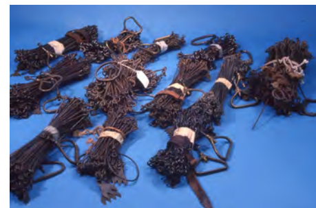
An assortment of chains: Gunter’s Chain, 66 feet. A half-chain, 33 feet. Railroad or Engineer’s Chain, 100 feet.
