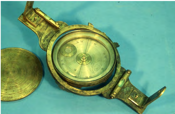
Gimbaled compass by James Reed (1792 - 1878) of Pittsburgh. Used in the mines.
