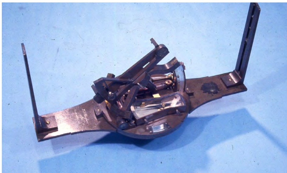
A rare Solar Compass by a very rare maker, John S. Hougham; Franklin, IN. Compass was made about 1861.
