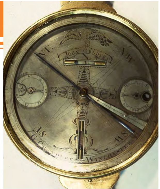
The face of a Goldsmith Chandlee (1751 - 1821) vernier compass; Winchester, VA, circa 1800. Eagle holding banner with "John Orndorf" for whom the compass was made.
