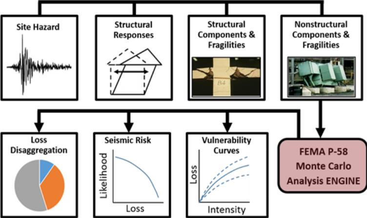
Figure 1. Outline of the FEMA P-58 seismic risk assessment methodology (Wade et al., 2018).
