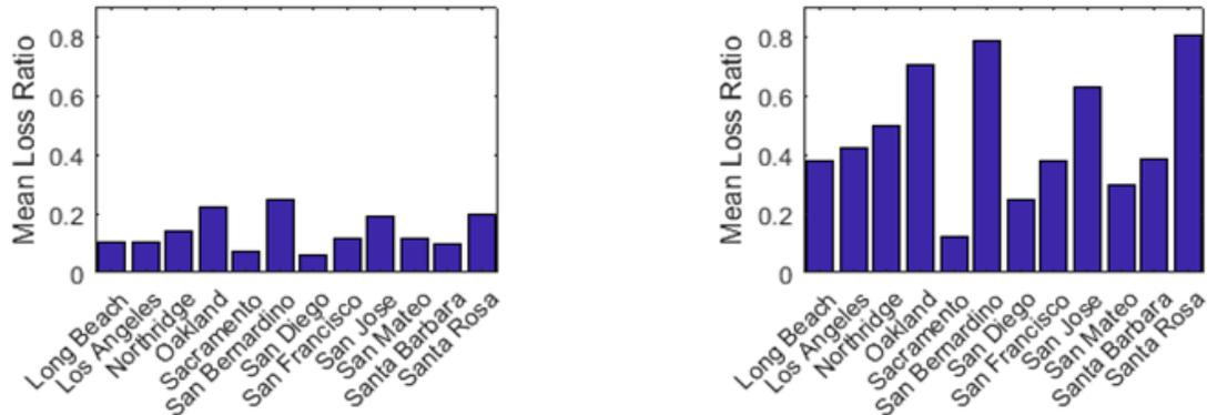
Figure 2. Expected repair cost normalized by building replacement cost for an 8-story steel moment frame building (a) 475-year event, (b) 2475-year event (results from a study conducted using SP3).
