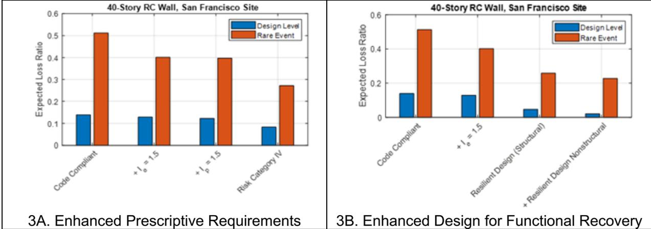
Figure 3. Expected performance for a 40-story reinforced concrete shear wall building with enhanced design requirements (Haselton et al., 2019)
