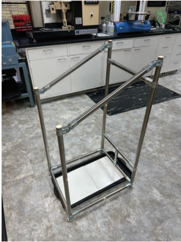
Figure 7. Metal handrail fixture.
