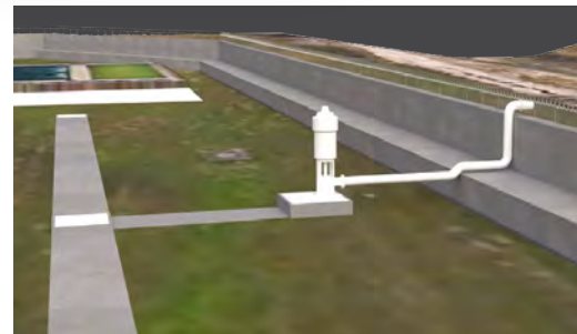
DRAINAGE PUMP AND SUMP
