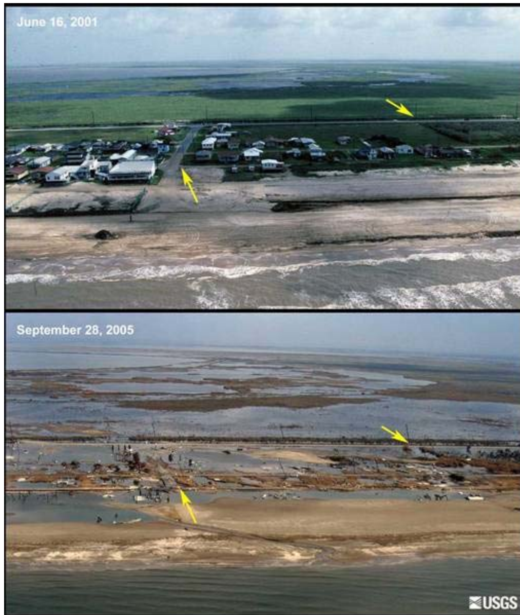
Figure 9: Aerial before and after images of Holly Beach, Louisiana showing the complete destruction of structures along the coastline. This area went through the eastern eyewall and suffered a storm surge of 15-18 ft resulting in total devastation. Source USGS
