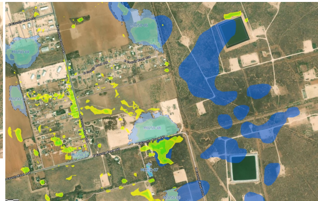
FIS floodplain (dark blue) denotes closed contours, but many do not capture runoff due to sandy soils or lack of contributing watershed.
