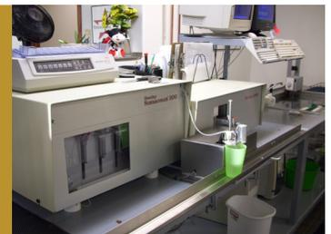
These results are entered in a spreadsheet which calculates the accuracy of the results compared to the "true" standard value. The fat and protein results must be within a margin of +/- 0.04, and lactose and other solids or SNF must be within +/- 0.06. If the results are not in the acceptable range, we may re-run samples, have the machine recalibrated, or try other samples.
