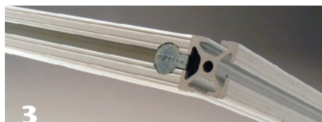
Special anchors join the four pieces of the frame. Order the horizontal pieces counterbored for the round part of the anchor.
