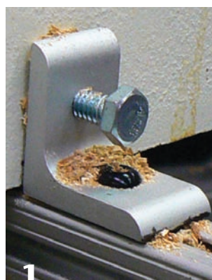
1 Arms on the frame have angle brackets that hold the shield in place against the lathe bed.
